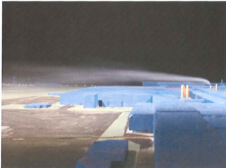
Figure 16. Photographs of selected exhaust plume flow visualizations for stack S_349: a) site structures in place for a wind direction of 100 degrees; b) site structures in place for a wind direction of 140 degrees.
