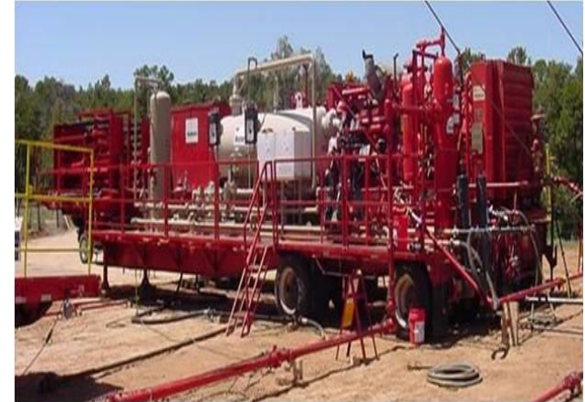
Green Completion Equipment (Source: Weatherford)
