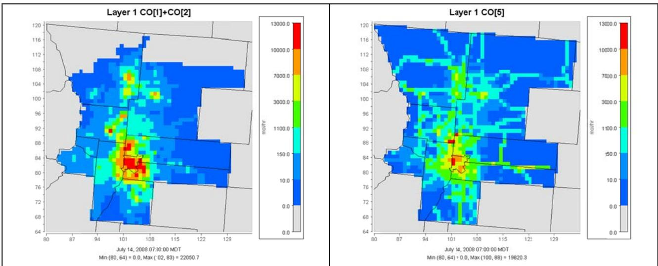
**Figure 5.** Off-Network start exhaust carbon monoxide (CO) emissions, July 14, 2008, 7AM MDT estimated by CONCEPT (left) and SMOKE (right).
