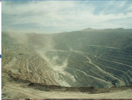
Removal of overburden
