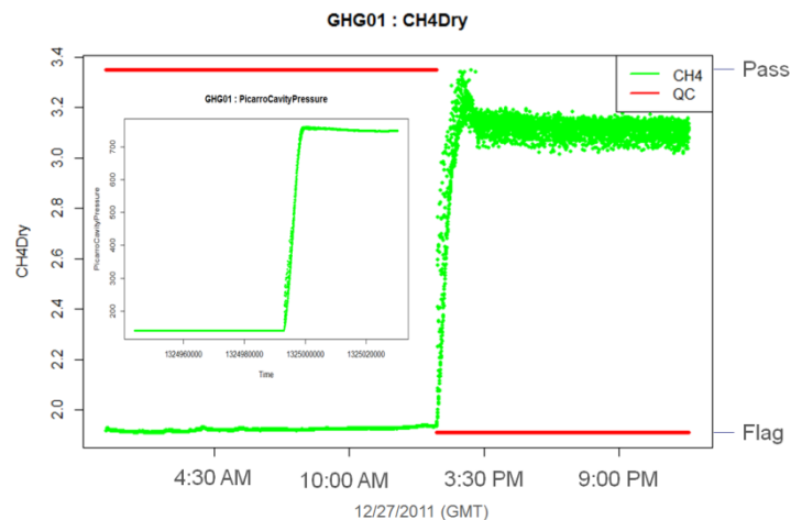
Figure 4. Example of data quality application to pump failure at GHG01.
