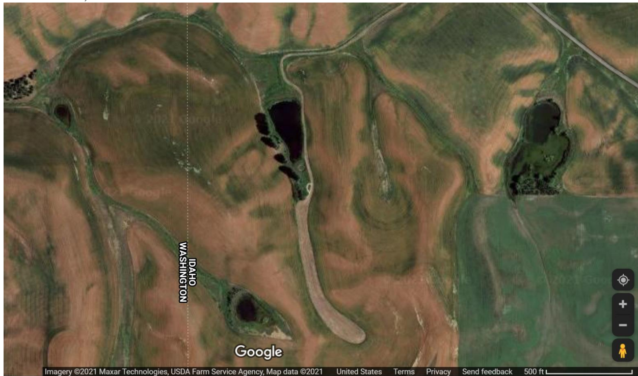
Photo 7 An aerial image showing four sediment basins designed to hold a permanent pool of water. Credit: Google Maps Imagery.
