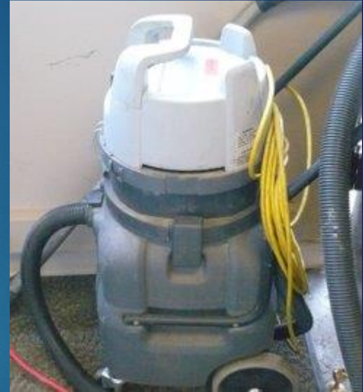
HEPA vacuum used to pick up loose paint chips outside
