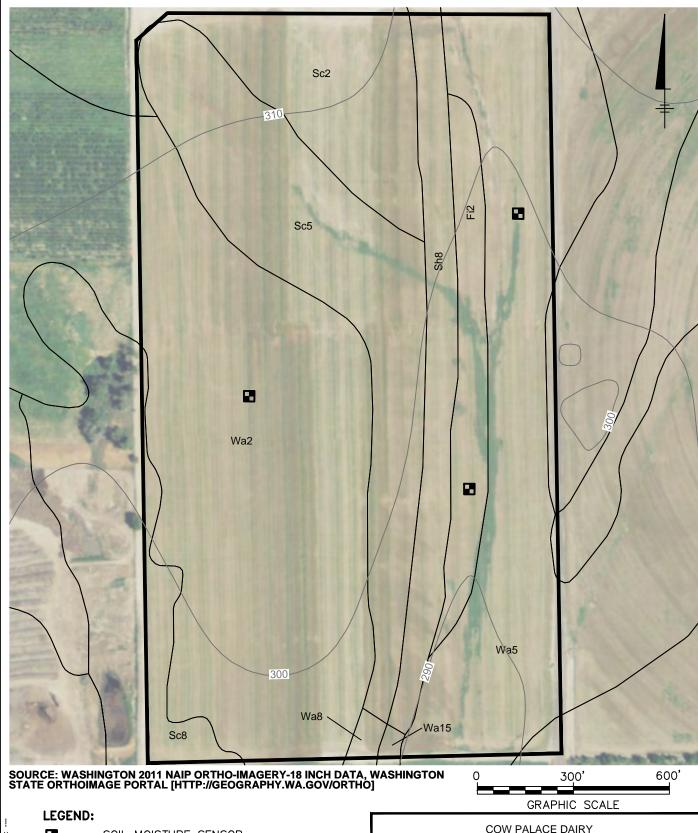
SOIL MOISTURE SENSOR 300-TOPOGRAPHIC CONTOUR LINE FINLEY SILT LOAM, 2 SCOON SILT LOAM, 2 SCOON SILT LOAM, 5 Fi2 TO 5% SLOPES Sc2 TO 5% SLOPES TO 8% SLOPES Sc5 SCOON SILT LOAM, 8 TO 15% SLOPES Sc8 - SHANO SILT LOAM, 8 TO 15% SLOPES
