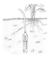
The sensor may be difficult to insert into extremely compact or dry soil. If you have difficulty inserting the sensor, try loosening the soil somewhat or wetting the soil. *Never pound it in!*
