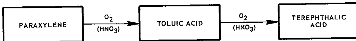
Figure 7-4. Terephthalic acid synthesis.
