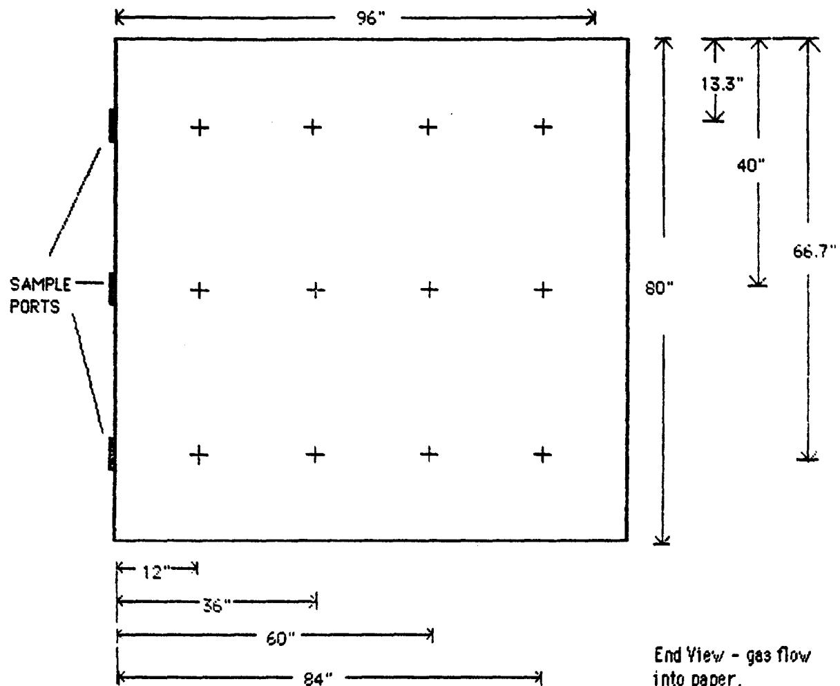
Figure 4 - Traverse Point Locations for Inlet Duct
