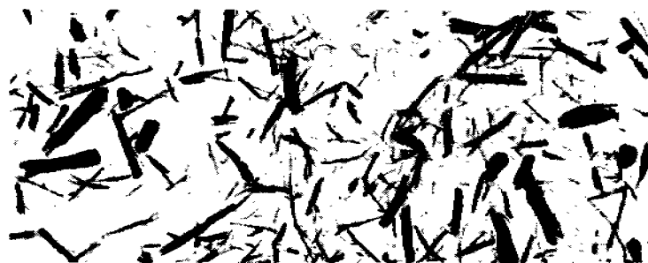
Figure 7.17. Dry-process fiber from cold refined shavings and sawdust; magnification 6 X (Rauch and Cheney 1970).
