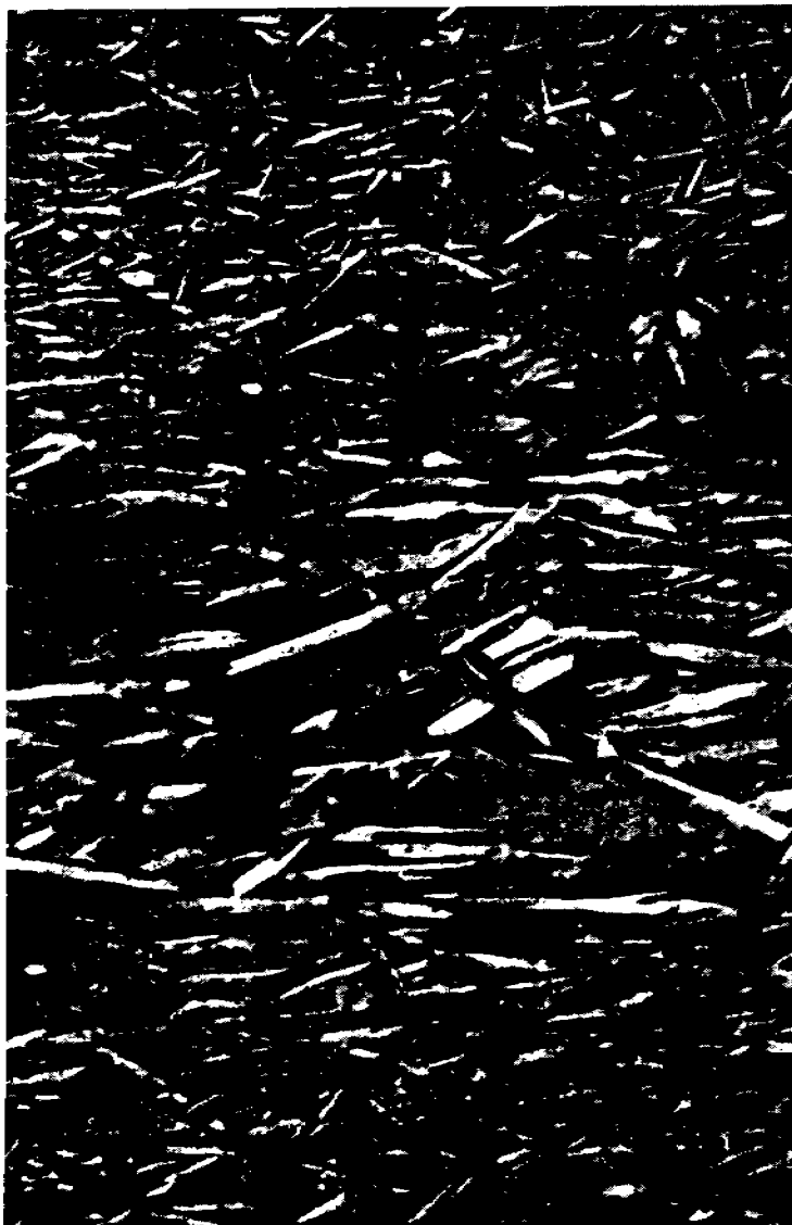
Figure 3.1. A graduated particleboard mat with fine face particles and coarse core particles (Haigh 1967).
