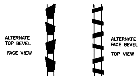
Figure 18.15. The alternate top bevel and face bevel tooth form used to prevent edge breakout (Kovich 1972).
