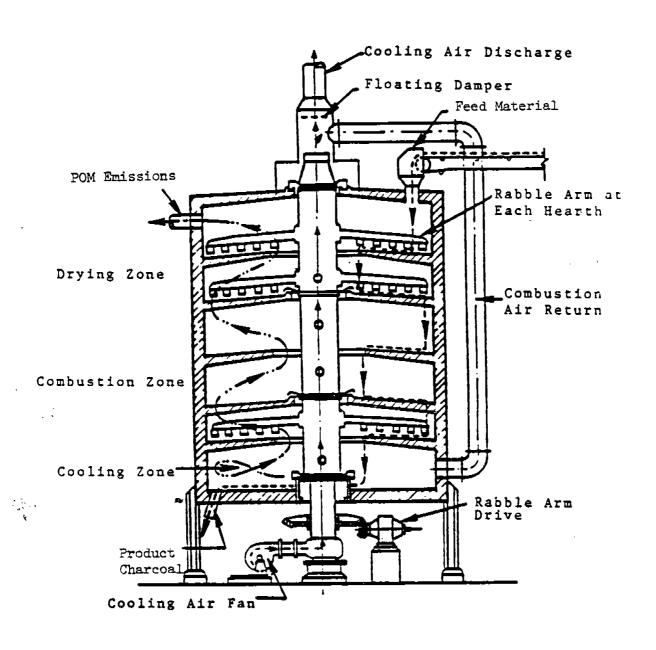
Figure 36. Multiple-hearth furnace for charcoal production. 148
