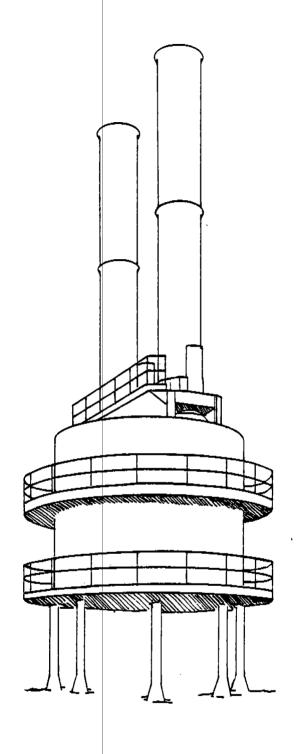
Figure 2-3. Exterior View of a Herreshoff Multiple Hearth Furnace.
