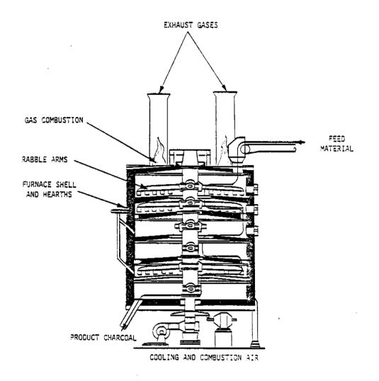
Figure 2-4. Cross Sectional View of a Herreshoff Multiple Hearth furnace.
