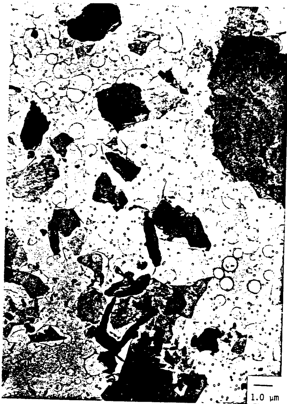
Transmission electron micrograph showing typical particulate matter found in water suspension after laboratory exfoliation of Sample 427-0, Grace, Enoree, South Carolina, Grade 5 (composite).
