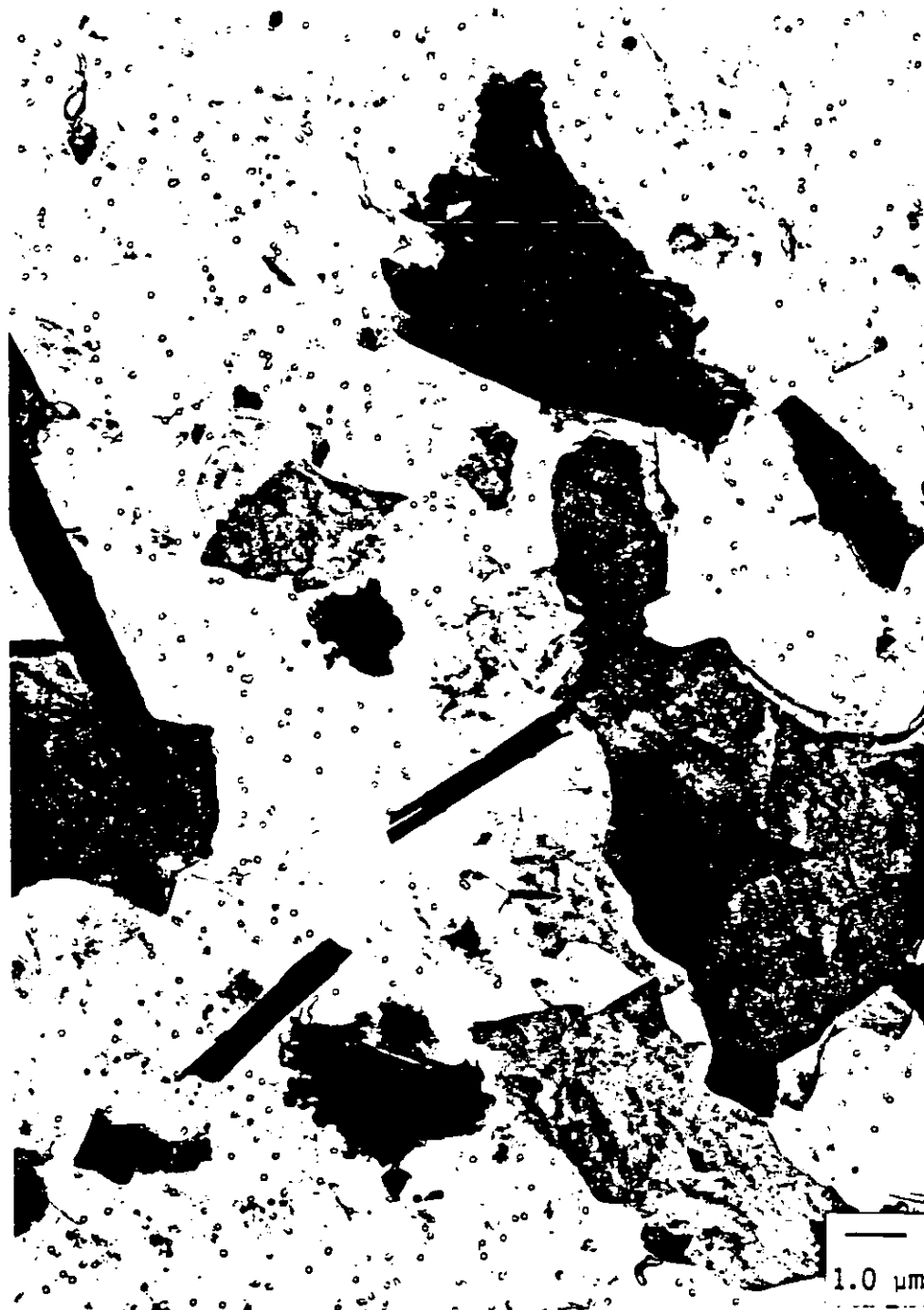
Transmission electron micrograph showing typical particulate matter found in water suspension after laboratory exfoliation of Sample 264-O, Grace, Libby, Montana, Grade 5 (composite).
