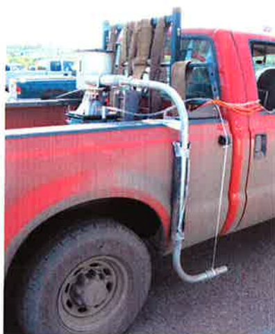
Figures A-5 and A-6. Views of the Mobile Monitor Intake Tube and Cyclone Pre-collector (left view) for Removal of Particles Larger than PM-10
