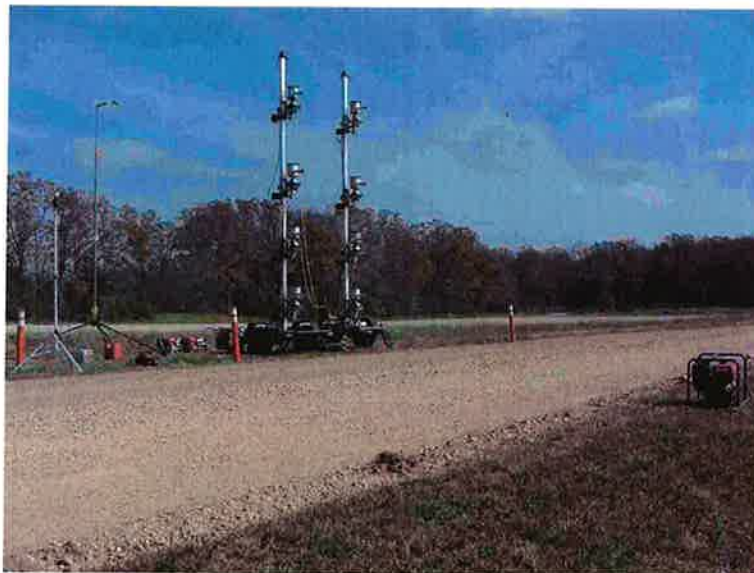
Figure A-1. Deployment of Co-Located Profiling Towers for Replicability Testing
