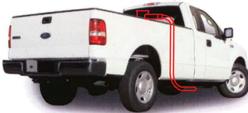
Figure 3. Mobile Monitor Intake Line on Side of Test Vehicle
