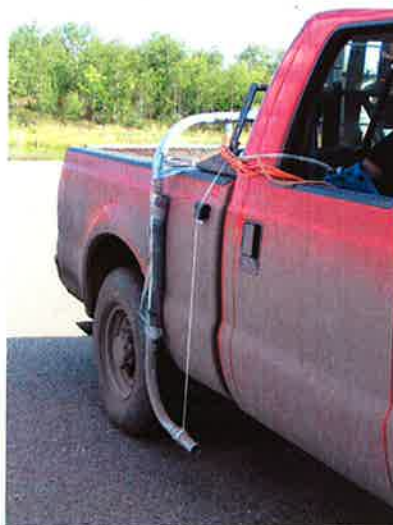
Figures A-5 and A-6. Views of the Mobile Monitor Intake Tube and Cyclone Pre-collector (left view) for Removal of Particles Larger than PM-10
