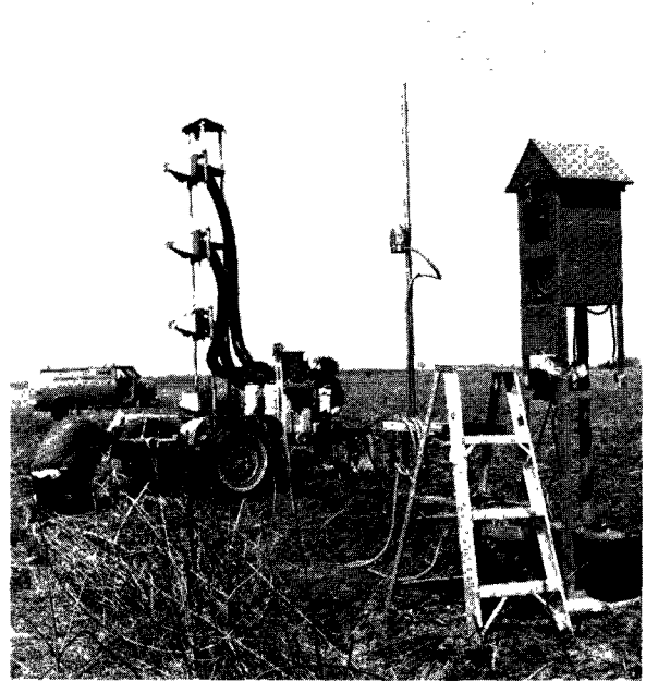
Plume Sampling Equipment
