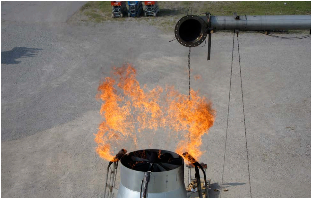
Figure B-8. Air Flare tip with vent gas separators.
