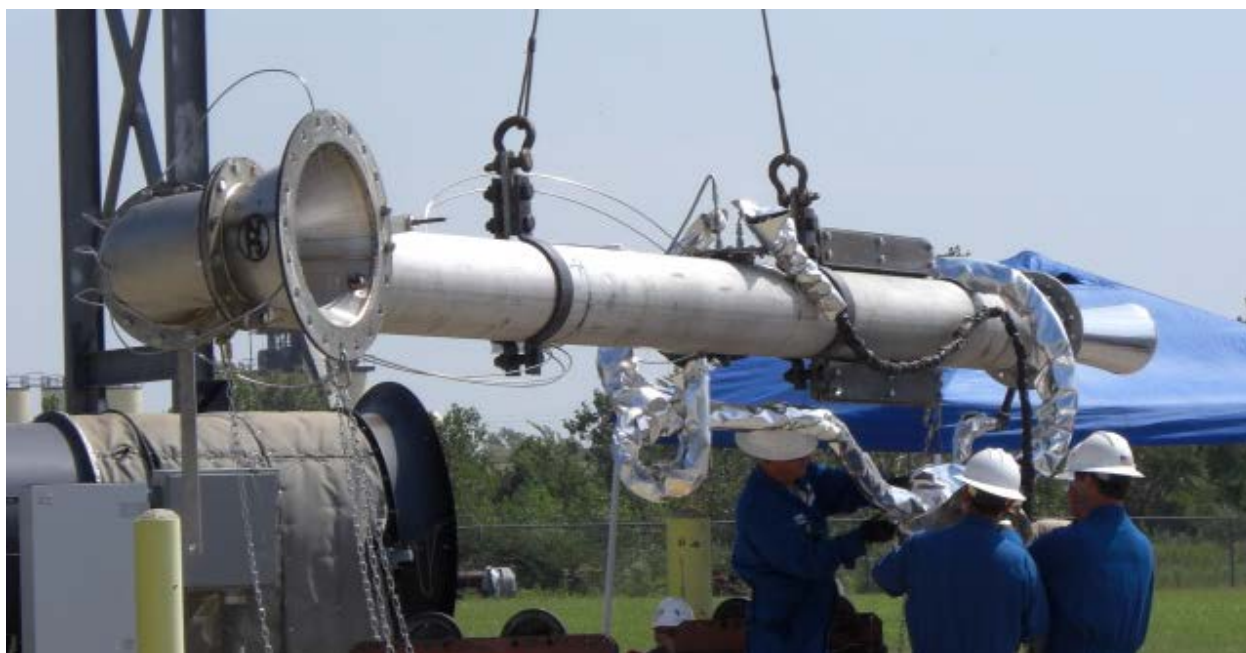
Figure B-14. Sample Collector at Near Ground Level – Collector inlet is at foreground and eductor is at far end. In photo, Zink personnel make adjustments to heated transfer line supports. Shackles and cable at center allow crane to lift and position Sample Collector.
