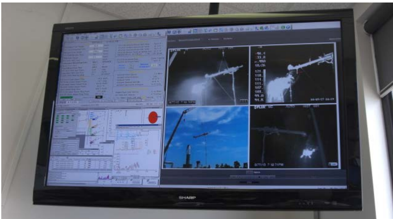
Figure B-12. Monitor in Control Room displaying Zink measurement of flare operating parameters (top left), LSI's FLIR and IR video (right half) and ARI's flare emissions measurements (bottom left)
