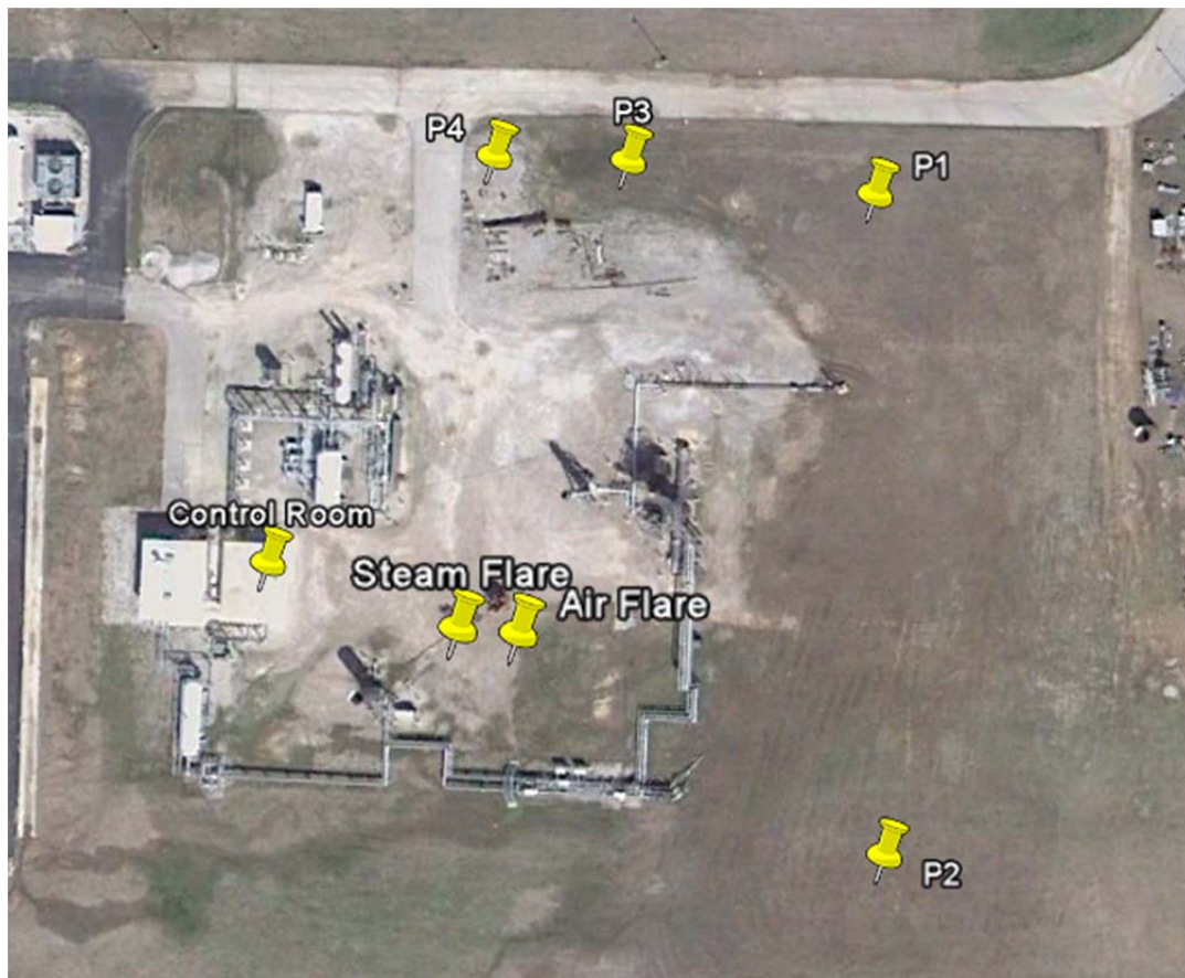
Figure 1 Aerial view of the John Zink test facility (taken from Google Earth). Pins labeled P1 to P4 indicate the location of Telops' sensor during the measurement campaign.
