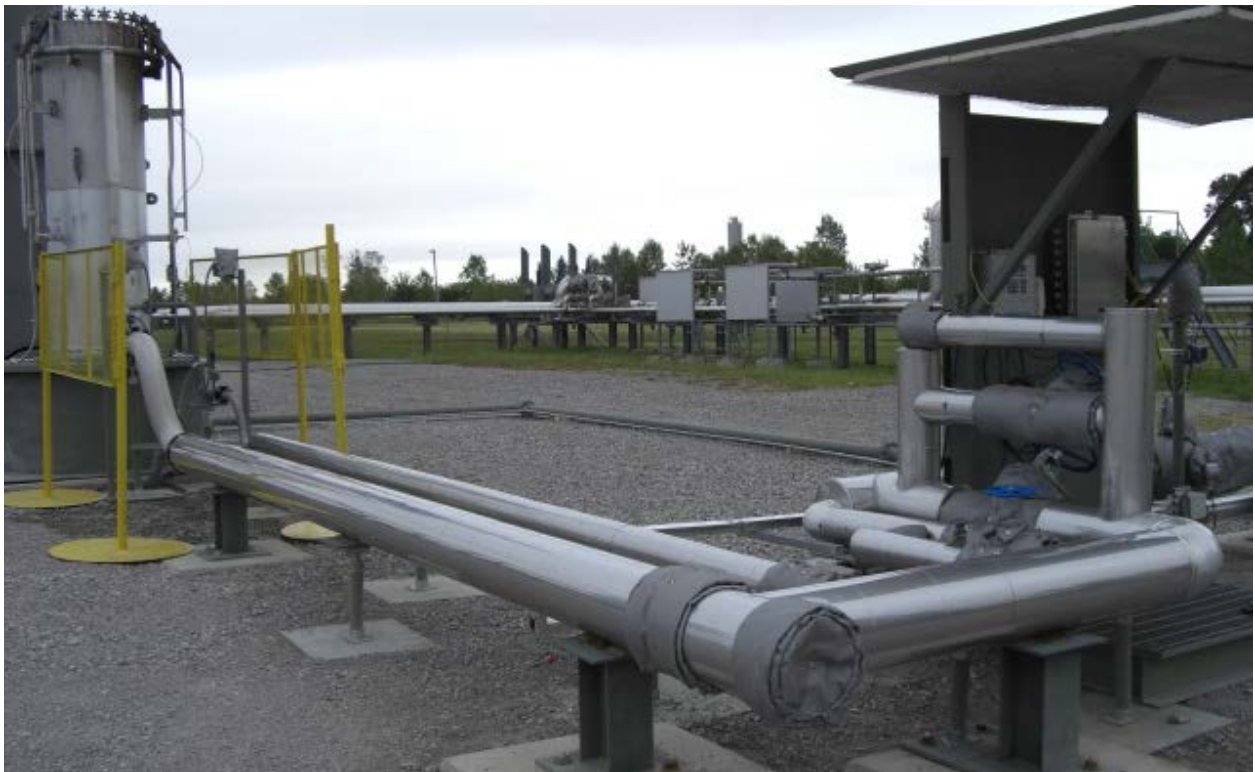
Figure B-5. Steam-assisted flare burner with upper steam assist line on left and center steam assist line on right. Steam control station is to the right of the steam lines.
