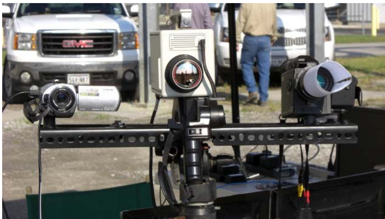
Figure B-15. Sony Handycam – for visible light (left), thermal infrared – for heat (center), and GasFind infrared – for hydrocarbons (right) cameras
