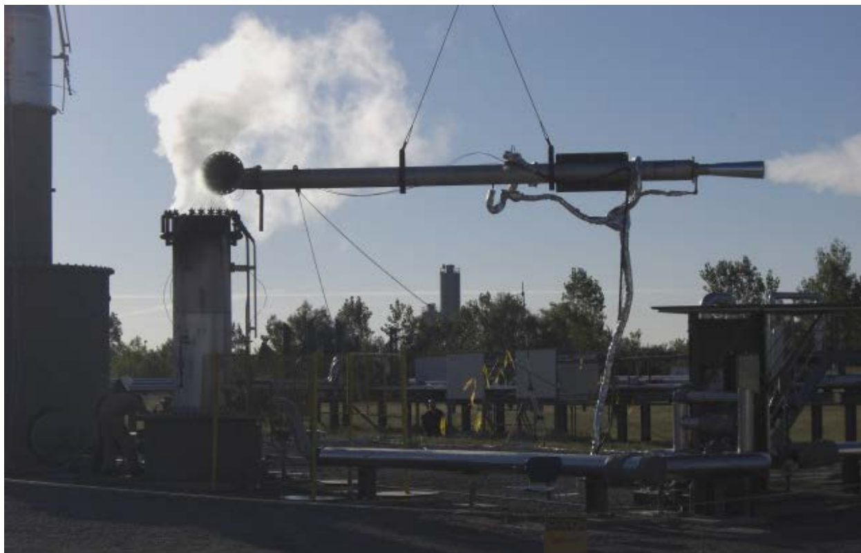
Figure B-2. Flare Plume Sampling System During Morning Start-up Routine
