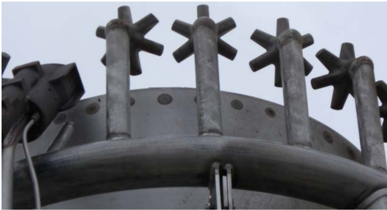
Figure B- 6. Typical pilot (left) and upper steam ring with nozzles.
