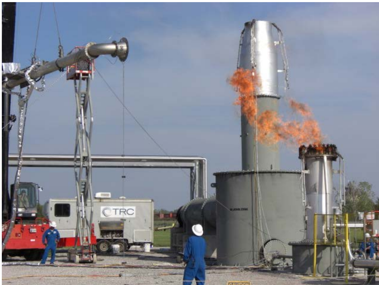
Figure B-13. Flare Plume Sampling System making measurements of flare plume while held in position by crane and ground crew.
