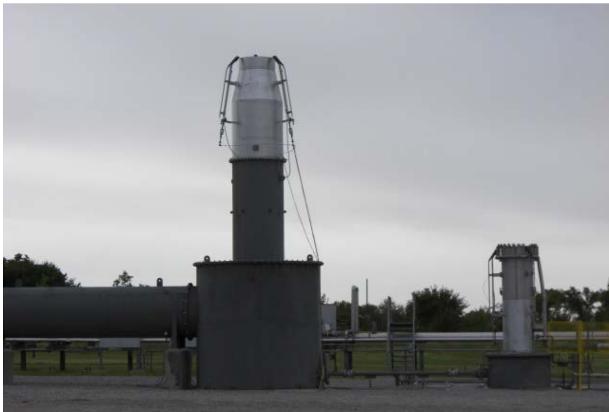
Figure B-3. Flare Burners – Air-assisted on left and steam-assisted on right
