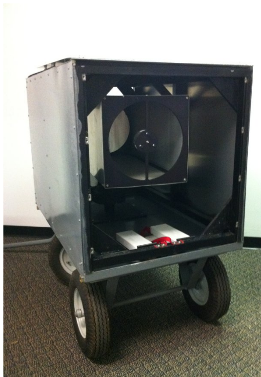
Figure 1 Imacc Source Collimator for Calibration of the PFTIR.
