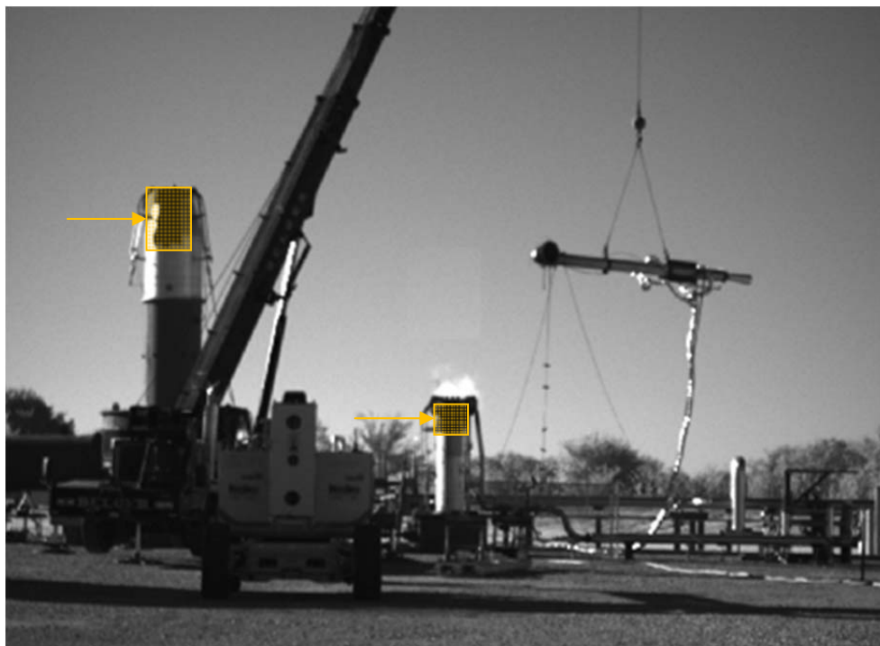
Figure 3 Air-assisted flare (left) and steam-assisted flare (center) illustrating the black painted area.
