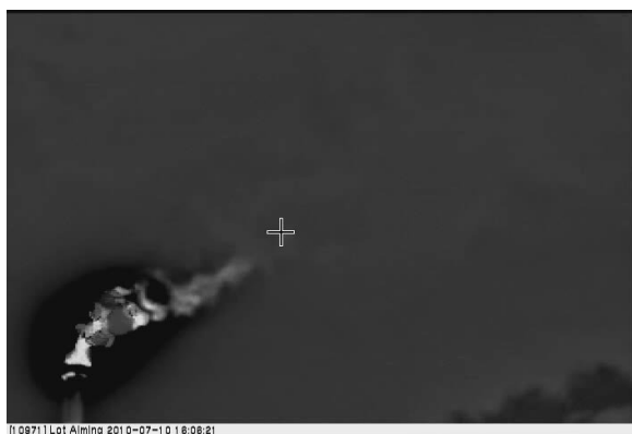
Figure 3.4-16: Aiming Camera with Good Plume Alignment
