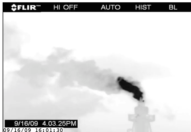
Figure 2.5-3: Image from FLIR GasFind IR LW Camera
