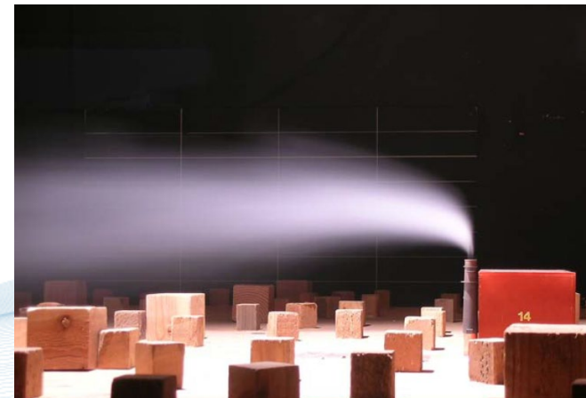
Figure 10. Vertical concentration profiles for isolated stack. In this and following legends, H_e/H_b identifies the presumed effective stack height as determined from analysis of vertical concentration profiles at position, x/H_b (see table 3).
