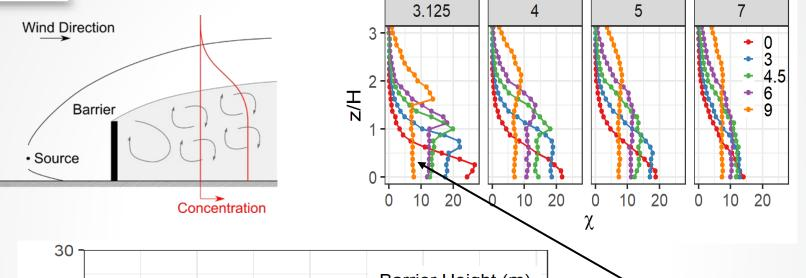
Vertical concentration profiles downwind of barrier
