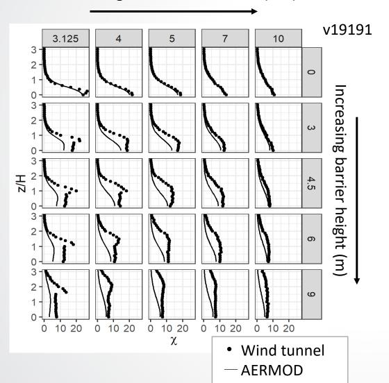
Vertical concentration profiles using barrier algorithm in AERMOD v19191
